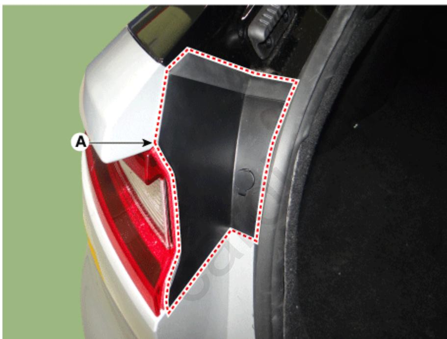
3. Remove the rear combination lamp (A) after loosening the mounting nut and screw.
