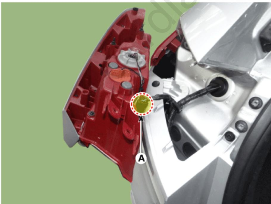
5. Remove the rear combination lamp deflector (A).
