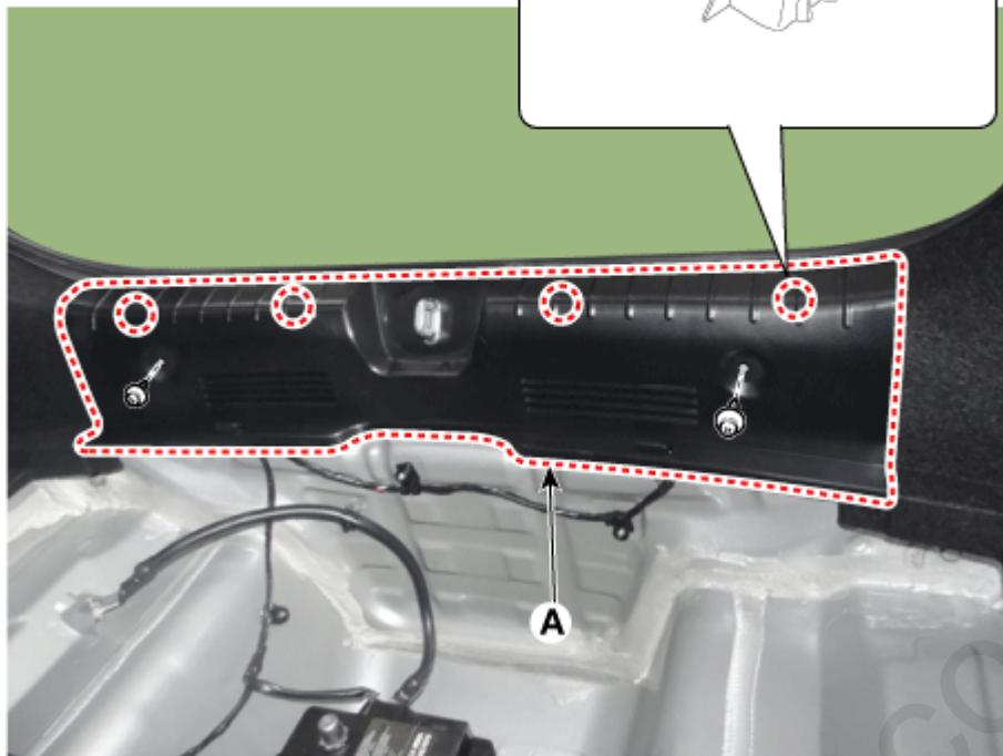
12. Separate the luggage side trim (A) after loosening the mounting screws.
