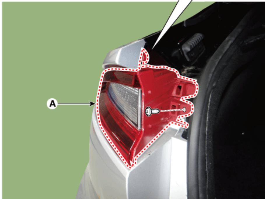
4. Disconnect the rear combination lamp connector (A).
